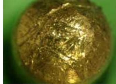
This is a very skilled attacker who uses extremely light tension and picking force to reduce forensic evidence. Despite skill, we still find similar forensic evidence. In this photo, pick marks are extremely light but still visible in the center of the pin. We can also see some marks on the side of the pin which are more defined.
