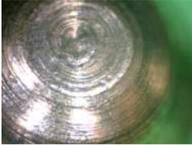
Up close we can see that the ring is actually due to the milling marks starting to be removed and lightly polished. The pin has also been slightly distorted in the very center, also due to the key making contact with it.
