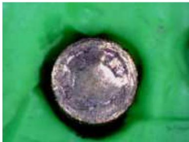
In some pin designs the bottoms of the top pins will be considerably damaged by bumping. In this case, the bottom pins are lightly rounded on both sides, allowing them to be inserted either way. When bumped repeatedly, the bottoms of the top pin become considerably dented.
