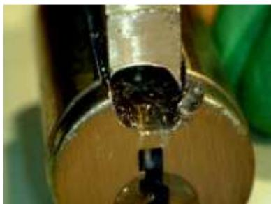
Drilling, a form of shearing, is the most common method of destructive entry against all types of locks. It is frequently used by locksmiths to remove locks when they cannot be opened non-destructively. In this photo, the plug of a KIK cylinder has been drilled at the shear line, allowing the plug to freely rotate.
