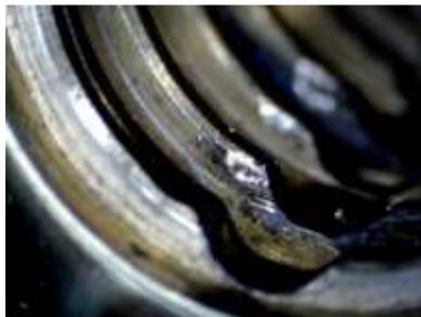
In this photo we see the cylinder from the failed bumping of an EVVA 3KS. The serious damage to the walls of the cylinder is due to the wafers slamming against the cylinder when bumping was attempted.
