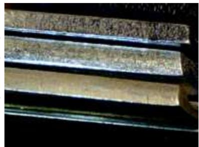
The plating on a key also provides some clues. Manufacturers usually plate factory-original keys *after* they are cut, while locksmiths and hardware stores will remove the plating of a blank key when making cuts. The plating material may also be used to identify the key blank manufacturer.
