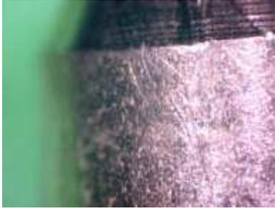
For the attacker, it is difficult to not touch the sides of pins. This can happen during raking as well as single-pin picking. Marks left on the sides of pins are quite noticeable and not as prone to wear and those in the center of the pin. In the photo, light scratches at varied angles are visible.
