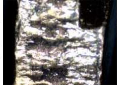
Of course, the plug and the top pins have continued to wear, with more brass being polished off and more pronounced staggering of the lubricant along the sides of the plug.
