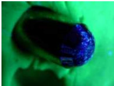
When using UV impressioning, UV ink is reapplied each time the blank is filed. In turn, the pins will have a large amount of UV residue on them. Notice the obvious key pattern of UV ink across the sides of the pin. In addition, the UV pen fibers may have been stuck to the key and left behind on the pins or the plug walls.
