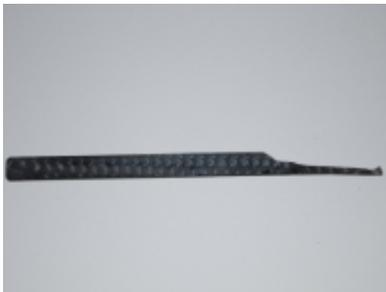
Carbon fiber lockpicks were considered for use in Anti-Forensics, but my research shows that they leave marks similar to traditional metal lockpicking tools. The photo shows a finished carbon fiber lockpick in the half-diamond design. This pick is roughly 0.025" thick.
