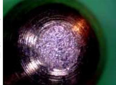
Constant movement of the vibrational pick gun needle causes numerous tool marks on the plug walls, as well. In this photo, various vertical scratches are present throughout the length of the plug. Some vibration picks also leave a stuttered or angled type of tool mark on the plug walls.
