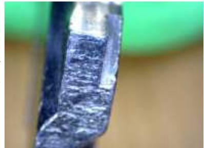
The face of the plug is also clean on a new lock. There should be few scratches or dents and little dirt or corrosion. The keyway material is not damaged, and the material just inside the keyway should not have any markings.
