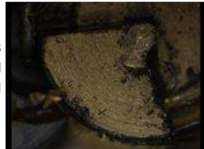
In response to the above attack American Lock (now owned by Master Lock) issued a hardware patch to prevent the bypass method. It is just a small metal disc, and in the photo we can see tool marks from where bypass was attempted. The 700 has since been redesigned because another attack against this component makes bypass again possible.
