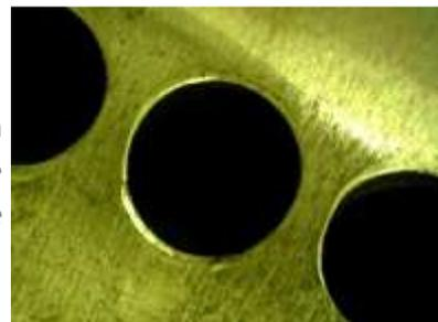
One of the most noticeable pieces of evidence from key bumping is damage to the face of the lock. This is caused by the shoulder of the key impacting the area above and below the keyway. The use of modified shoulders may prevent this from happening, see the [Anti-Forensics](#) page.
