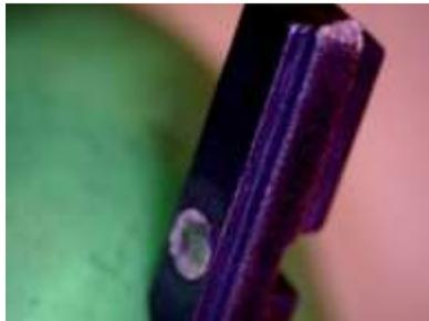
Many unskilled attackers may attempt to bump unbumpable locks. This will probably damage the lock and borders on breaking the lock completely. In the photo, an EVVA 3KS wafer is shown after an bumping attempt. The wafer arm has broken off and a large dent is present, this lock was non-functional after this.
