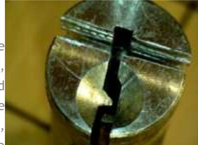
not cut down the middle as may be expected (see photo). Cutting into thirds is preferred over halves because the top portion of the keyway is never touched by components, including the key, and is considered virgin territory where forensic evidence may be present. See the [lockpicking](#) page for more information of possible marks in this area. To cut the plug, a fine-tooth hacksaw or jeweler's saw is used.
