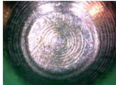
There are many other designs of pin-tumbler besides the standard round or pointed tips. This is a photo of a Mul-T-Lock telescoping pin tumbler that uses an inner and outer pin stack. Both show signs of picking tools. If we separate the pins, we would also probably find picking marks on the inside chamber of the outer pin.
