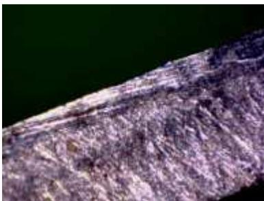
When a key is duplicated with a stylus-based key machine a mark is left on the side of the original key. This is due to the stylus being gently dragged against the key, and resembles a long, straight, polished line. This cannot be confused with wear of the key because it is not in the direct center of the key.
