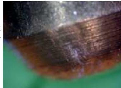
Like carbon fiber picks, fiberglass does a very good job of trapping trace evidence from the pin-tumbler inside the lock onto the pick. In this photo, the tip of the fiberglass pick is shown with light brass residue and lubricant (black) clearly visible.
