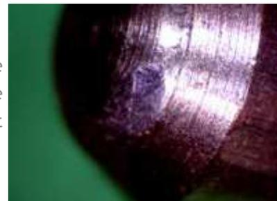
Alternate lighting may be used to illuminate bumping scratches and dents more efficiently. In this photo, there are dents on the left, center, and top of the pin, as well as scratches. In many cases it is possible to count the number of times the bump key was used by counting the dents.
