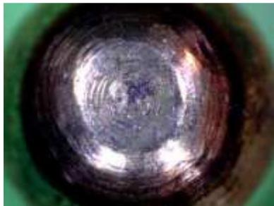
Compared to other pins, pin 5 (the farthest back) continues to show reduced signs of wear and retain its milling marks. We can also now see that wear is not evenly distributed on this pin, as it resembles an oval shape. Compare with above picture and 1,500 use pictures.
