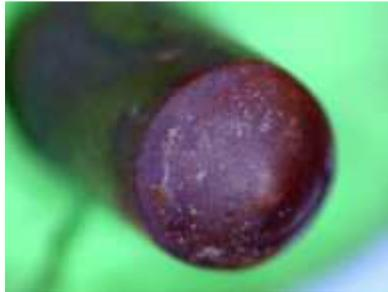
Chemicals are powerful because they can fundamentally alter metals to leave them vulnerable to many other attacks. In this case, brass pins are dark red/brown because of  $\text{NO}_2$  fumes released when concentrated nitric acid contacted the brass components. Nitric acid has the effect of eating away the copper in brass.
