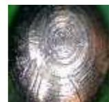
This photo is similar to the last, but instead there are many varied, elongated scratches at different angles and depths on the pin. This type of marking is indicative of a pick that is designed to be gently rubbed against the pins at varying height and tension. Of course, this is the technique known as raking or rake picking.
