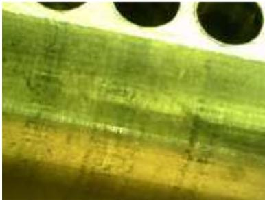
The plug is also showing signs of wear, caused by the top pins gently rubbing against it when the cylinder is turned. (Note: The top pins also show signs of wear because of this, but I have left them out to keep our examination simple.)
