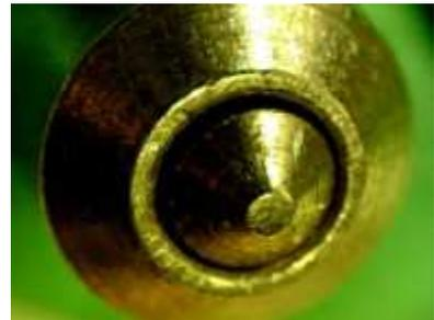
Some pin tumbler designs are rather strange, designed to deter manipulation. This photo shows a Vachette VIP "nippled" pin. The design of this pin is rather complex, with not only a nipples tip but also a very spool like appearance. In any event, picking marks are visible along the nipple and base of the pin.
