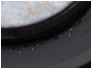
The Code Lock (4000 series) electromechanical lock is subject to a bypass attack that manipulates the bolt actuator. In the photo, material has been removed from both the actuator and the tool (a thin piece of metal) and scattered around the inside of the lock.
