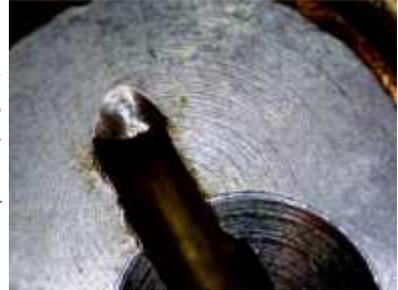
In the minimal-movement method, material is removed from the tip and shoulder. This makes the method work but also inserts the key far enough that in some cases affects the keyway. This is due to the key material getting thicker as it reaches the bow. In the photo, this can be seen around the edge of the keyway.
