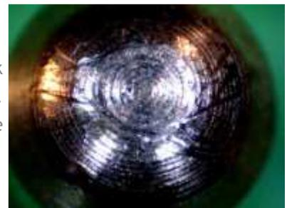
After 250 uses (roughly 2-4 months use) the tip of the pin has been worn by the key, leaving fewer distinct picking marks. At the same time, the sides of the pin still show very clear and distinct picking marks. This is because the key does not touch these areas as frequently and may never, depending on the key biting.
