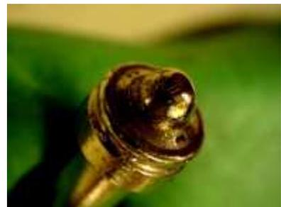
Forensic evidence is also left behind by various lock-specific tools, which are growing more common with high-security locks. In this photo, the pick marks from a Medecoder type tool are visible in the sidebar channel where the tool was used to rotate the bottom pin.
