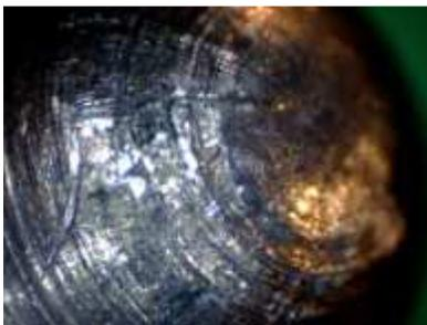
Carbon fiber picks did not work as well as I had hoped. Most importantly they fell short of surreptitious by leaving marks on pin-tumblers similar to traditional tools. In this photo, light scratching along the tip and side of the pin can be seen, caused by a carbon fiber lockpicking tool.
