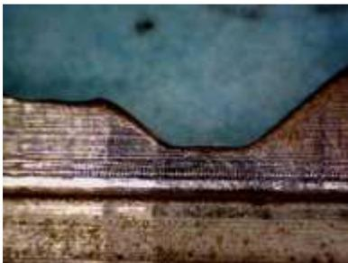
In this photo, the duplicate key is shown. Notice that the ramps and valleys of the key are slightly different than the previous photo. In addition, we see that the key is nickel-silver plated, with no plating on the cuts. Depending on the factory-original specifics, this may also indicate that it is a duplicate key.
