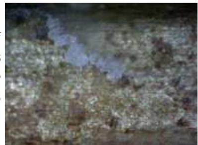
Keys should also be viewed under various light sources to attempt and find any material residue that may not be visible with the naked eye (or naked microscope?). In this photo, a key is being viewed under ultraviolet light to discover traces of ultraviolet ink along the key biting area, indicative of impressioning via manipulation.
