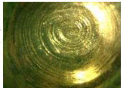
The key continues to wear and collect lubricant. Image shown at high zoom to show the literal pits that are being created. At this point, certain ramps on the key may be acting like a file when going in and out of the lock. As seen above, this translates to more light scratches on the tips of the pins.
