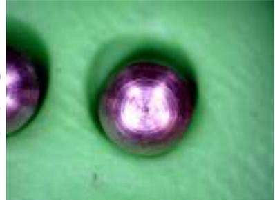
Up close, we notice many small imperfections in the tip of the pin. Very light scratches, dents, and bumps are visible. The dents and bumps are natural imperfections in the manufacturing process, while the light scratches are likely from the use of a key.
