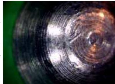
The marks left by a pick gun are so distinct, compared to the rest of the pin, that it is often possible to count them to determine how many times the pick gun was triggered. Each time the needle strikes, the bottom pins may rotate slightly, allowing marks to be separate and distinct.
