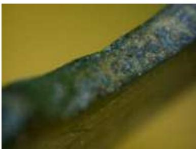
Carbon fiber lockpicks also seem to grab and hold pin materials much better than their metal counterparts. In the photo, a carbon fiber pick is shown with brass residue from the pins of a lock it has picked. This can be used in court as evidence to link a suspect to a crime.
