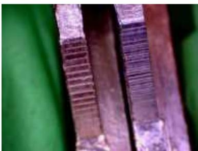
Keys can be examined to determine the speed and blade design of the key machine was used to cut them. This photo shows a comparison of two keys, with the one of the left being cut with a lower speed key cutter. If a key machine is found with a suspect, it can be examined to determine if it was used to cut a specific key.
