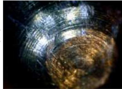
Fiberglass is also less surreptitious than carbon fiber because the act of picking and raking the lock leaves behind a sizeable amount of fiberglass on the pin-tumblers and walls of the plug. In this photo, fiberglass residue can be seen on the tip of the pin-tumbler.
