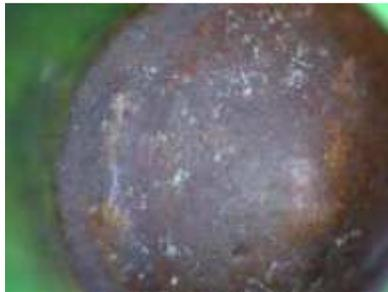
A closer examination can confirm the use of nitric acid by identifying trace evidence left by the chemical reaction between nitric acid and brass. The scattered blue particles are cupric nitrate and zinc nitrate, a byproduct of the chemical reaction.
