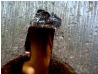
In shoulder stopped locks (almost all modern locks qualify), continued use will cause light impact marks along the face of the plug. This is normal, and should not be confused with the extreme material displacement that occurs during key bumping.
