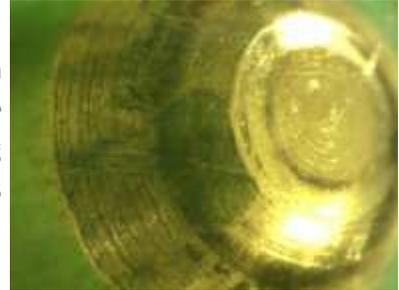
While taking the last photo I noticed a strange shape in the top right of the photo. When I refocused in that area I found this. It appears to be a small piece of brass that has transferred to the tip of the pin, probably a very small fragment of the key. Quick, call the crime lab!
