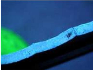
Keys that have been used in manipulation based impressing may show impressing marks along the key bitting. Close examination of the key for such marks may help to determine its intended purpose. In the photo, an impressing mark is found by viewing the key under ultraviolet light.
