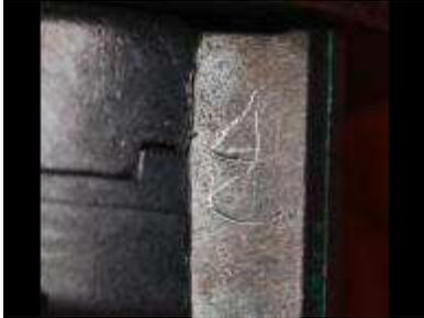
In most forms of bypass that target the actuator, tool marks on the actuator are distinct. In this photo, we see tool marks on the actuator of a Code Lock (4000 series). Notice tool marks are at a variety of angles and depths, all of which are inconsistent with normal use or wear.
