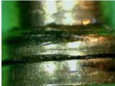
Bumping is rarely 100% successful, either because bottom pins are bumped above shear line, or top pins are not bumped high enough. When this happens the tension applied will misfire, causing one or more top pins to bind. This causes light shearing against the bottom of the top pins.
