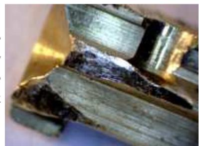
The pins in simulated lockpicking will have a large amount of material removal and tool marks that are not consistent with any type of covert entry, including lockpicking or key bumping. Marks will usually not be found on the pins in the back of the lock, too.
