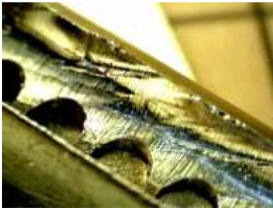
Drills are much like firearms in terms of forensic evidence. Bullets fired from a gun have striae based on the barrel used; the same goes for drill bits used in destructive entry. In the photo, the spiral striae left by the drill bit can clearly be seen in the plug of the lock.
