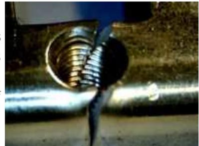
The basis of this attack is that there is enough of the cylinder extending through the door, as little as a few millimeters, and a tool used to grab and apply force to the lock. In this photo, tool marks can be seen where the tool was used to grab the front of the lock.
