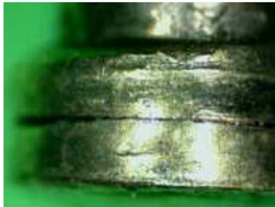
Some top pin designs will be more affected by bumping than others. In this photo, a spool pin with serrated edges is shown. Repeated bumping of this pin has caused the serration to close up (compare with previous photo). In general, situations like this slightly decrease pick resistance.
