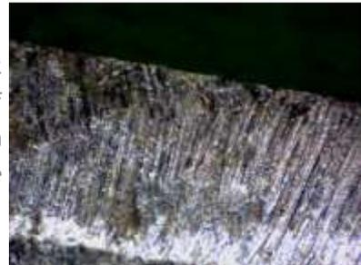
In this photo we see a series of cuts with variable depth valleys and light material removal around the edges. This is consistent with use of a dremel. Again, tool mark comparison can determine exactly which dremel bit(s) may have been used. These can be linked with tools found in a suspect's possessions.
