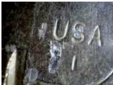
Sometimes marks will be left on the key as a result of normal or malicious use. When a key is duplicated with a cutter, the clamp to hold the original or the blank may leave a mark. In addition, some covert entry techniques may leave tool marks. In this photo we see a set of rather deep marks on the bow of the key.
