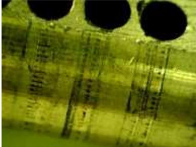
At 5,000 uses the plug continues to show increased wear, though not much has changed. More pronounced staggering of wear and lubricant can be seen along the circumference of the plug. Compare with example at 1,500 uses.
