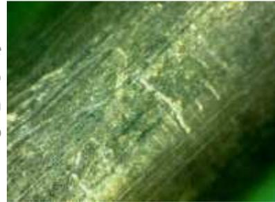
Sometimes, impressioning marks are so clear that we can count the rounds of impressioning. If marks are far apart the forensic locksmith can also measure the distance between them. This may indicate a more skilled attacker if they are using factory depth increments to speed up the impressioning process.
