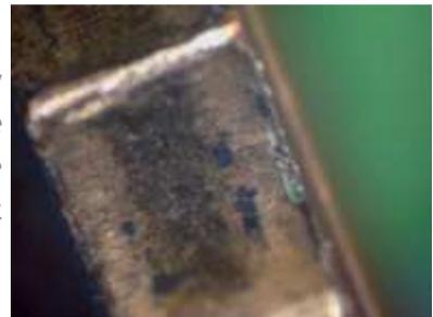
In this photo we find small traces of white wax left in the warding of the key. Both this and the previous image indicate that the key has been impressed (via copying). Through further analysis we may be able to link these and other materials to those found in a suspect's possessions.
