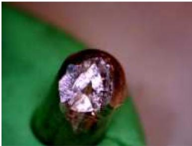
The pins inside this lock show heavy damage from where the screwdriver or chisel was forced into the keyway. Examination of what is left of the tip of the pin shows no indication of covert entry techniques. Because of the force used, tool marks on the pins are rather distinct and may later be used to link suspects to the crime.
