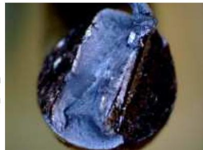
A closer examination of the tool mark reveals that a red substance is present in the area where the bolt cutter was used. This could be a variety of things; paint, dirt, grease, or rust. We might be able to match this material to the tool if a bolt cutter is found in a suspect's possessions.
