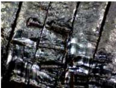
A closer inspection of the tool mark shows a series of parallel teeth marks, probably from the use of a plumber's wrench or tongue-and-groove pliers. Marks can be used in tool mark comparisons done with tools found in a suspect's possessions.
