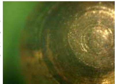
What is most interesting is that pin 5 (the furthest back) has considerably less wear, and more visible scratches. This all makes sense; it is only touched by the tip of the key, and the tip of the key is the most worn down because it makes contact with all of the pins.
