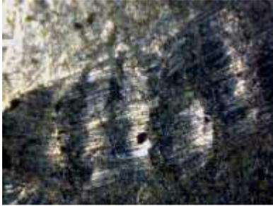
Close up we see a distinct pattern on the largest tool mark. We can hypothesize what made this, and perform a tool mark comparison to confirm. This particular mark was made by a pair of vice grips being used to impression (via manipulation) a blank key. The key should also be examined for impressing marks.
