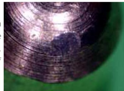
A bump key that is cut by hand, with a low speed key cutter, or made of a considerably stronger material (steel, iron, nickel-silver) than the pins may act as a file as it impacts bottom pins. In this photo, light scratches can be seen traveling through the bumping dent.
