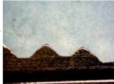
In this photo we see many groups of scratches, with slightly different angles, across the bitting of the key. This is consistent with the use of a file. Specifically, this is a flat file being used on the broad side. With a tool mark comparison we can determine the size, shape, and grade of the file(s) used.
