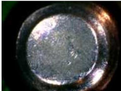
At 5,000 uses (roughly 5-6 years of use) the front pin has no milling marks, and almost all scratches have been polished away. From this point on wear looks similar to this, with light markings sometimes being created by wear of the key.
