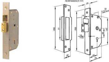
A key operated 5 detainer deadlock. Suitable for main entrance doors as well as inter-communicating doors.
