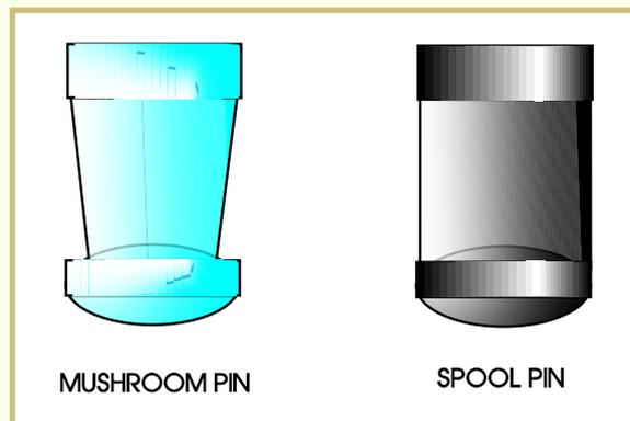
When you begin lifting such pins with a rake or feeler pick, they jam between the plug and the shell as shown in Figure 13.
