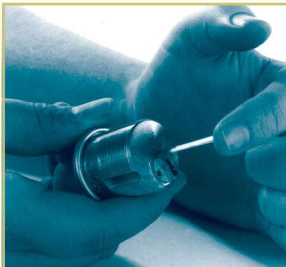
placed in the small gap between the plug and the cylinder. Once started, the shim is pressed into the cylinder until it strikes the first upper pin.
