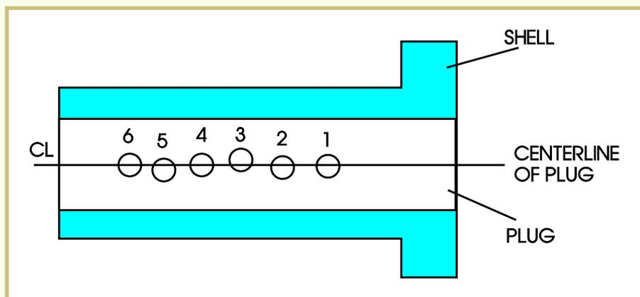
Since the holes aren't aligned, the short pin with the most clockwise offset will have the greatest force against it. Lifting this pin next will cause the plug to shift the greatest amount when the upper pin reaches the shearline. To continue picking the lock, try the remainder of the short pins; once again, lift the pin with the most tension. Continue this process until all the pins are lifted and the lock opens.
