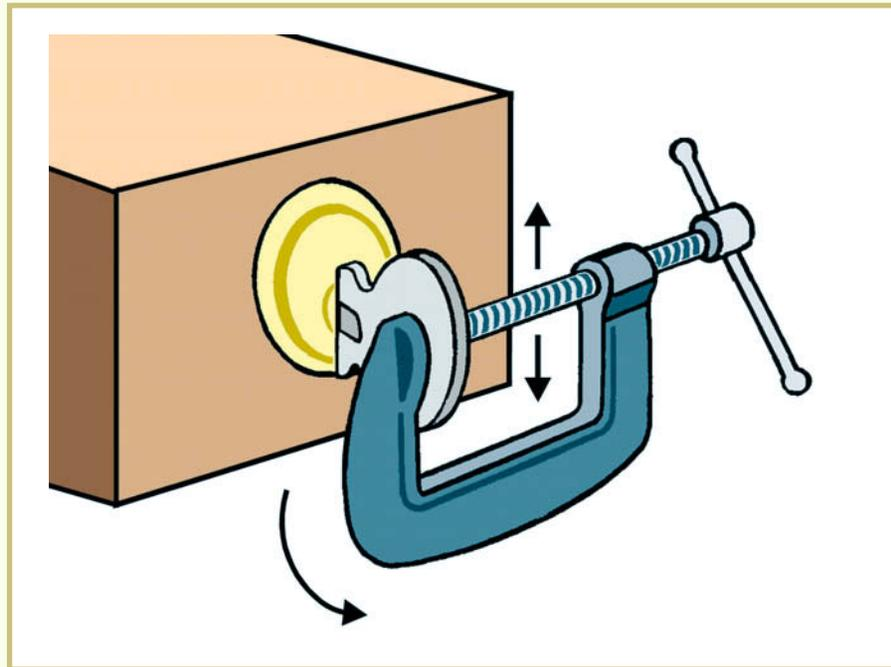
**Step 3:** Remove the key and examine the edge of the blade under a bright light. Rotate the key at an angle to help you see the impressions better. Seeing the impressions is often said to be the most difficult part of impressioning a key blank, so look very carefully. If you prepared the edge properly and moved the key correctly, you will see five slight impressions on the edge of the blade. If you didn't make impressions, re-read the instructions and try again.
