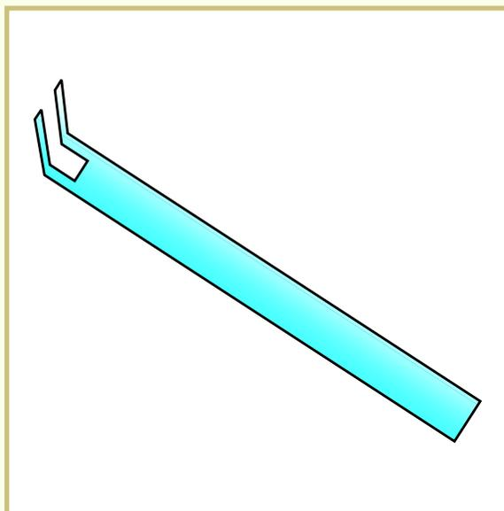
To pick this kind of lock, you'll need a double-sided tension wrench like the one shown in [Figure 9](#). This wrench is made of spring steel and has two tangs that enter the upper and lower side of the keyway.
