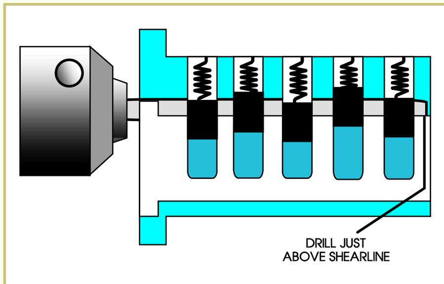
the lock as far as the key would enter, turn the plug with a tension wrench or screwdriver.
