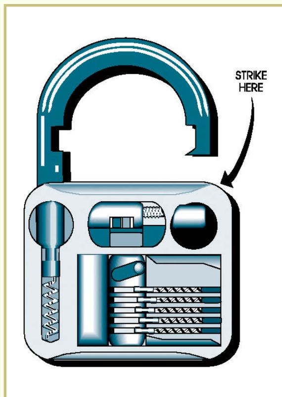
One brute force method often used by the nonprofessional is to use a long pointed bar or crowbar to slam the lock. Although this method is often successful on inexpensive padlocks and combination locks, it can damage the lock's shell, shackle, or locking mechanism.
