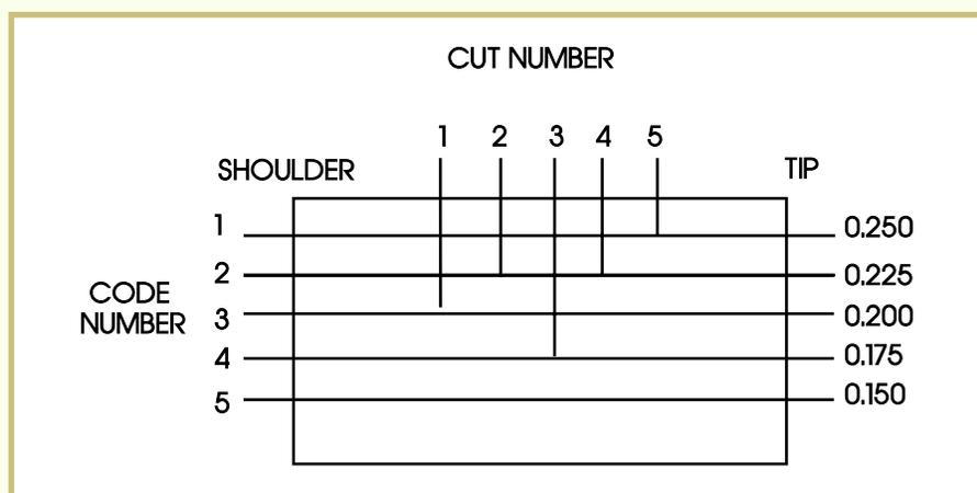
When reading a lock, the length of the first pin or slot size in a wafer or disk is a critical judgment, because all of the other codes are compared to this first wafer, disk, or pin. If you're off even by one code number, the entire code sequence will be off, also. In our example key code of 3, 2, 4, 2, 1, if you're off by one number on the fifth cut, the code might advance by one number, resulting in a key code of 4, 3, 5, 3, 2. As you can
