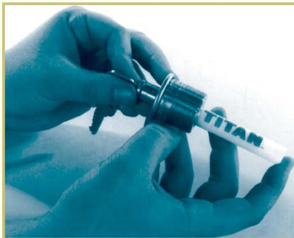
**Step 11:** Empty the lower pins from the plug. You are now ready to re-pin your lock. The pin combination that you must use is 31512. Select the proper pins from your *pinning kit* and place them in your plug in the proper order. You may want to measure the pins to be sure you are using the correct size. The proper length of each is marked in your kit. You can use a caliper, micrometer, or simply sort the six different sizes in your kit.
