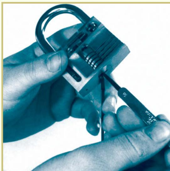
**Step 3:** Continue picking the cutaway lock until you get all of the tips of the lower pins at the shearline. Then, the tension wrench should open this lock.
