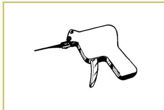
When the trigger is pulled, the pick is sprung upward within the plug, forcing the pins or disks upward. While the basic operation of a picking gun is simple, it takes practice to actually get one to open a lock!
