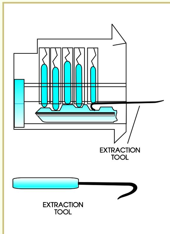
One problem that often occurs during impressing is key breakage. Normally, the key breaks at the blade's shoulder or just before it. When this happens, a simple extraction tool, such as the one shown in [Figure 26](#), can be used to grab the blank and pull it from the plug.
