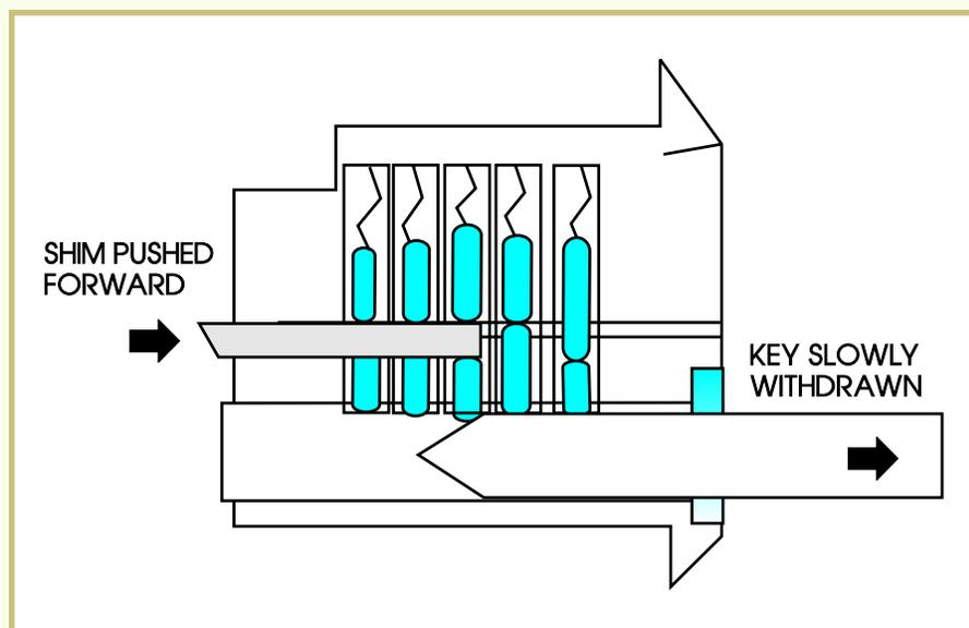
In practice, the shim is placed at the rear of the plug and the blank key is inserted into the front of the plug. This action will force most if not all of the lower pins into the shearline. As the key is slowly withdrawn, the lower pins will settle back into the plug. If the proper pressure is placed on the shim, it will separate the upper and lower pins as the lower pin rides down the angle of the front of the blank key's blade.
