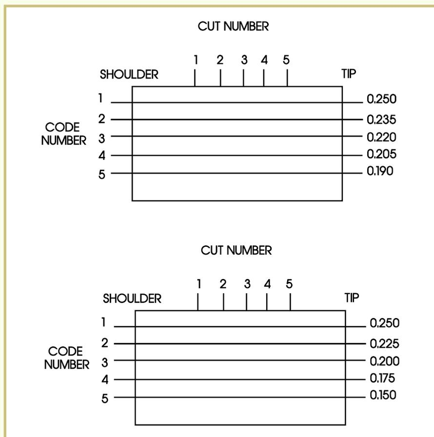
**FIGURE 29**—The reading chart shown here will display the cuts needed for a key for a lock coded 3, 2, 4, 2, 1.
