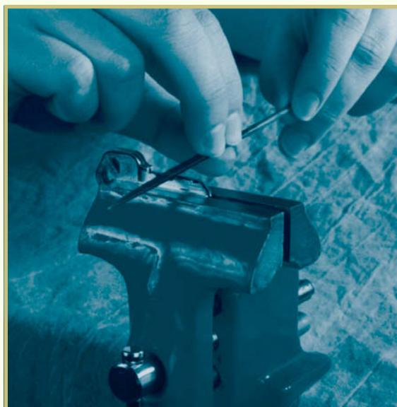
**Step 5:** Re-insert the blank in the lock and re-impression your key. Some locksmiths work on only one cut at a time. They repeat the impressioning process and deepening one cut until the pin no longer makes an impression at that location.
