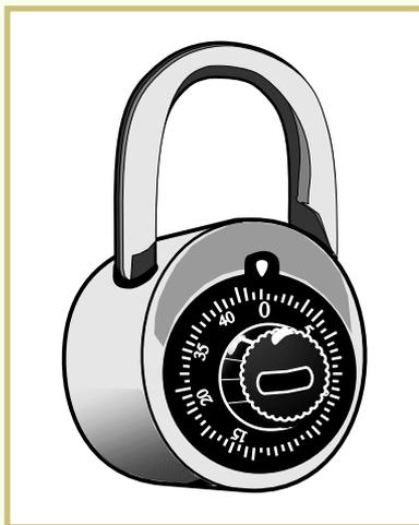
Once these numbers are “dialed,” an internal locking dog is released, opening the lock’s shackle. A typical combination padlock is shown in [Figure 19](#).
