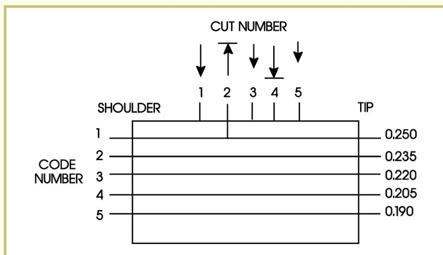
in the slot, meaning that this slot is in a number one disk. Now, the relationship of the disks is known, and you have a starting point for completing your reading chart. This chart is shown in [Figure 34](#) with a line drawn to the number one cut depth on the chart.
