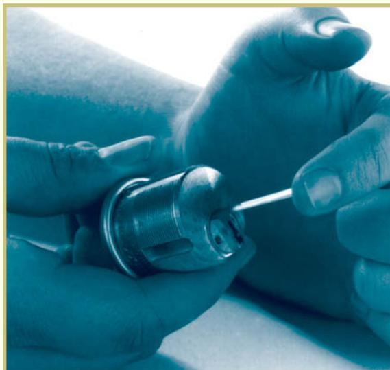
**Step 5:** With the shim in place, insert the feeler pick into the keyway of the mortise lock. Use the feeler pick just as if you were attempting to pick the lock with the feeler pick and tension wrench. However, go all the way back to the rear of the plug and lift the last lower pin.
