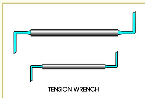
A tension wrench is made of spring steel, which allows for strength along with great flexibility. The blade of a tension wrench must be very thin (to fit in the keyway) yet be strong enough to apply the needed turning
