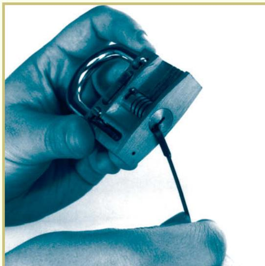
**Step 2:** Next, holding your feeler pick between your fingers like an ink pen, place it into the keyway. Feel the tension on each pin and begin picking the pin with the greatest tension on it. This procedure is shown in [Figure B](#).
