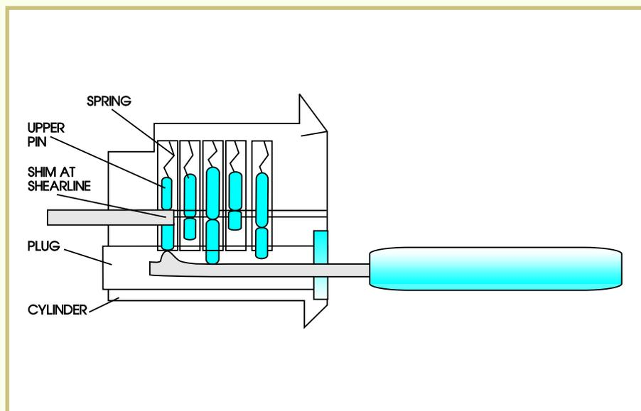
**Step 7:** With the shim seated against the second upper pin from the rear of the plug, pull back gently on the feeler pick until it strikes the lower pin. Now, carefully raise this pin with your pick until the shim slides gently forward. Don't apply too much force on the shim stock and bend it. Once bent, the shim stock will need to be removed from the lock and replaced.
