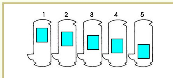
types of disks in the plug. These five disks are shown in [Figure 30](#). Note that the shape of each disk is identical. Because the key slots are positioned in different places on the disk, a different cut depth is required to lift each individual disk to the shearline, thus allowing the plug to rotate.
