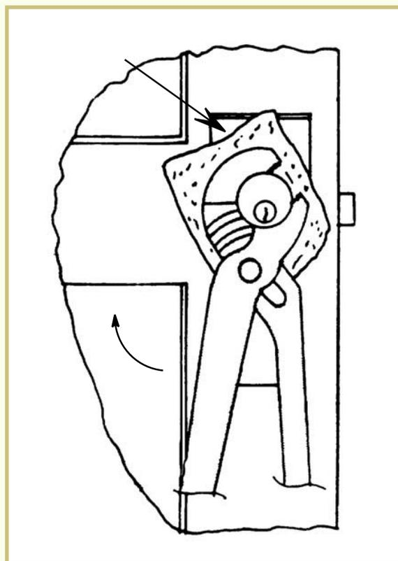
A soft cloth or a circle of plastic material can be cut to protect the door from damage.
