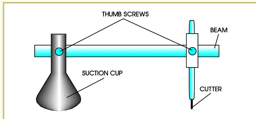
After this pass is complete, hold the suction cup on the glass and use a small pointed object to tap on the glass in a circular pattern where the glass has been scribed by the cutter. Normally, when you've tapped around the entire scribed circle, the glass circle can be lifted out with the suction cup.
