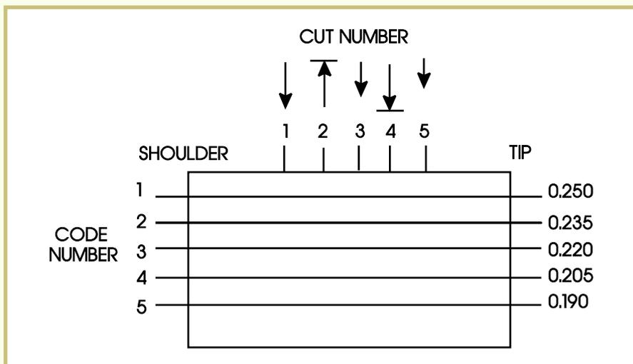
Remembering that a number one cut requires a full blade width of 0.250 or one-quarter inch, you can make a tool to read a number one disk. Simply bend a piece of wire at a right angle so that its small end is exactly one-quarter inch. Insert this wire into the plug of the lock. In our example, gage the height of the second disk. If the disk lifts, it will be a number two or three disk. In this case, the wire fits perfectly
