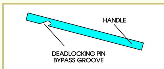
By wiggling the bar properly, you can move the latch behind the deadlocking pin and free the strike on the jamb.
