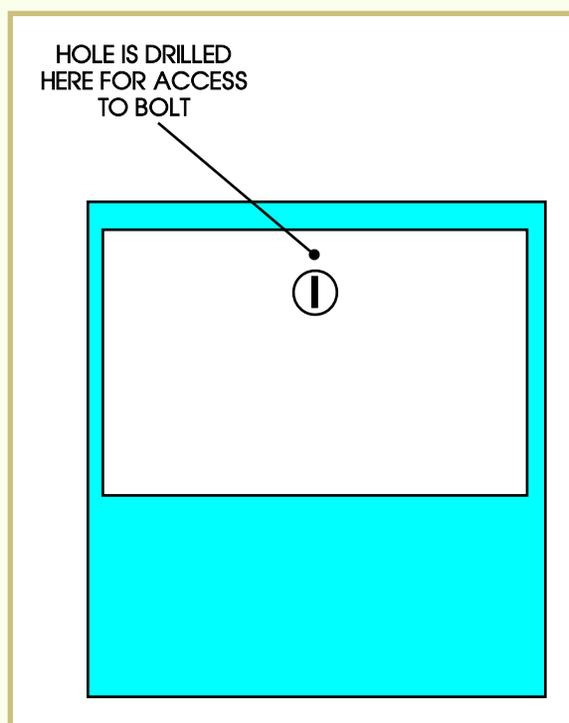
quickly and easily drill a hole of this diameter through wood or steel drawers without the need to run extension cords. Once the hole is drilled, you can insert a small, straight-pointed spring steel pick inside the hole. Push down on this pick while pulling gently outward on the drawer. The pick lowers the bolt, releasing the drawer. The hole can then be filled in
