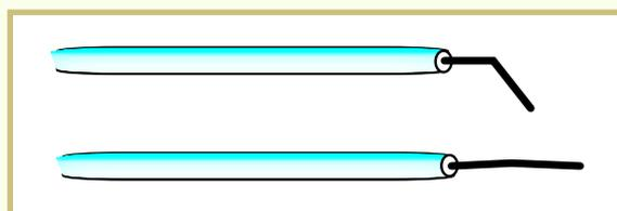
As you can see in [Figure 27](#), one type of reading tool has a straight pick end that's bent shortly below the handle.
