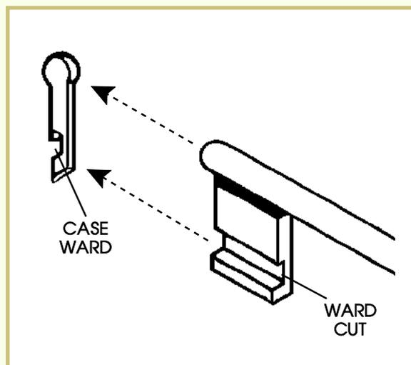
the blank's end with a candle. With a good layer of soot on the blank's end, press it against the cover ward and wiggle it slightly. Use a needle or scribe to draw two lines on the blank, one line just above and one line just below the case ward.
