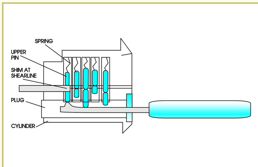
In this illustration, note how the shim holds the upper pin above the shearline of the plug. Also note that when you release the lower pin with your feeler pick, this pin will drop back down into the plug. The shim should have advanced into the cylinder until it strikes the next upper pin. Don't apply too much force on the shim to advance it. You don't want to bend the shim. If a shim is bent, it will require you to remove it from the lock and begin over with a new shim.
