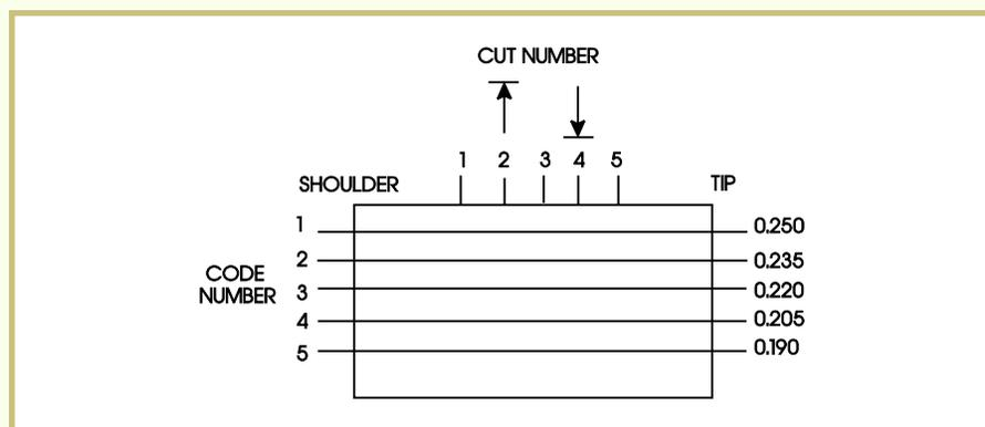
Note the use of arrows on the reading chart. In the case of this disk tumbler lock, the second cut from the key's shoulder has the smallest code number (shallowest key cut), while the fourth cut from the shoulder has the largest code number (deepest key cut).
