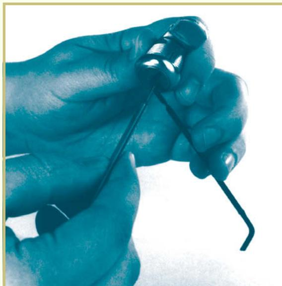
With the tension wrench in place, insert the rake pick just above the tension wrench (Figure 8). The rake pick should enter the keyway without lifting any disks. If it interferes with the disks, remove both the pick and the tension wrench, then replace the tension wrench at the top of the keyway.
