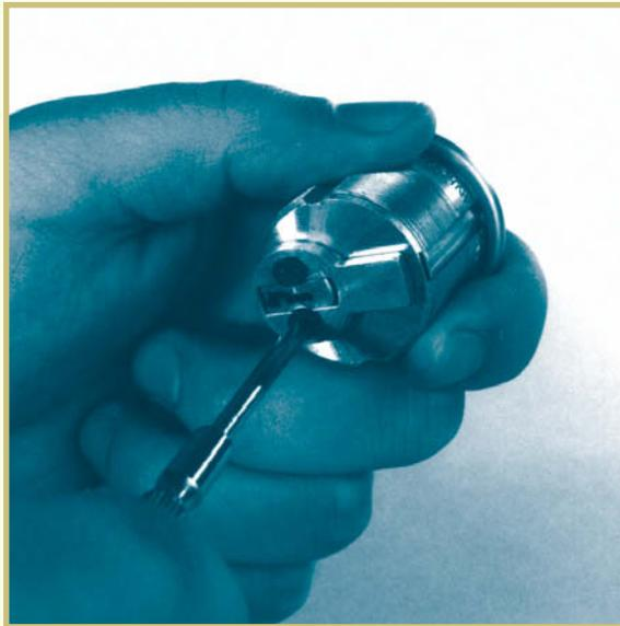
Two small screws are used to hold the retainer plate to the plug. Select a proper fitting screwdriver, remove these screws, and place them and the retaining plate in a tray or other container.
