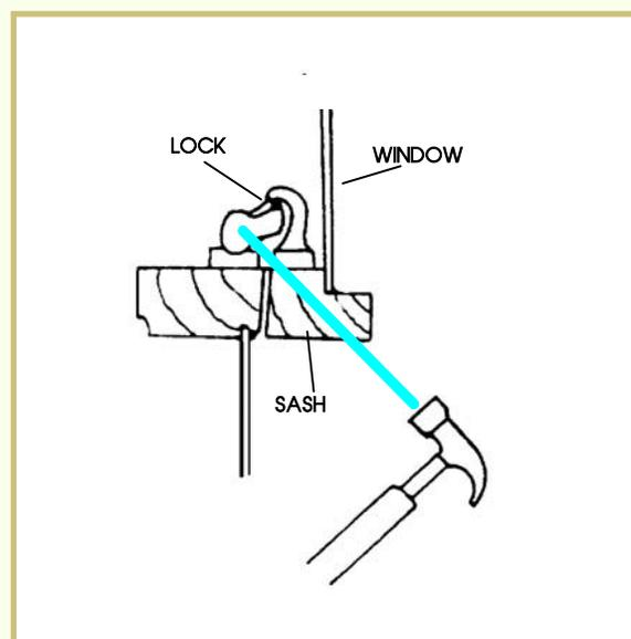
When drilling the hole, use a one-eighth inch drill bit. Place the hole in line with the latch handle. Once the hole is drilled, slip a piece of stiff wire or drill rod into the hole, until it contacts the latch handle. Then, tap the wire or rod with light blows of your hammer to open the latch.
