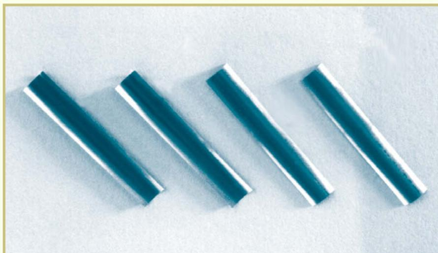
A shim can be used to open a pin tumbler lock, and are usually used to open mortise and rim cylinder locks. To do so, the shim is placed at the rear of the plug and pushed forward until it strikes the rear most upper pin. Then, a feeler pick or a blank key is used to raise the pin until it reaches the shearline where the shim is advanced to hold the upper pin above the shearline. Once all pins are separated by the shim, the plug can be turned and the lock opened.
