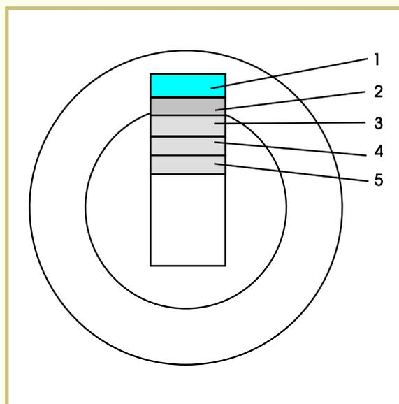
If the disks are placed in the plug in numerical order, the slot heights would appear as shown in [Figure 31](#). Since the dimension between the different code numbers is only 0.015 inch, only a slight amount of difference exists between the slot positions.
