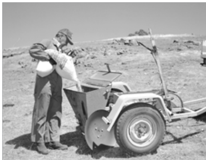
A bait layer being loaded for rabbit control
