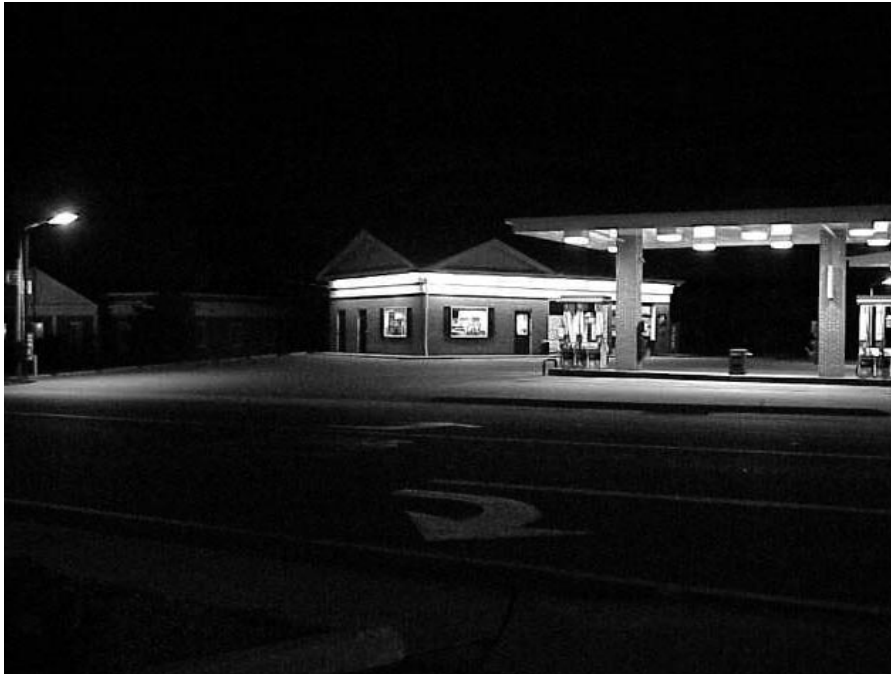
Figure 27 (a). Transition between pump island and service building is facilitated when uniformity ratios do not exceed 4:1. (Photo courtesy of General Electric.)
