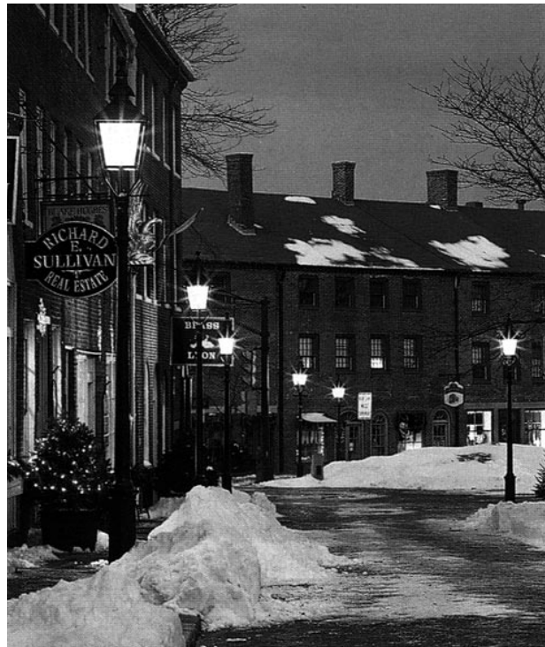
Figure 3. Pole-mounted "lantern-style" luminaires help create a turn-of-the-century theme for this street, which is home to numerous upscale businesses and stores. They are equally attractive during the day or night. Care should always be exercised in choosing decorative luminaires, which may produce glare and light trespass. (Photo courtesy of OSRAM SYLVANIA.)
