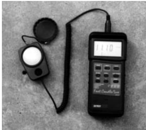
Figure C1. Typical illuminance meter. (Annex C photos courtesy of Operational Support Services, Inc.)
