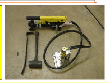
The Rabbit Tool is a handheld, manually operated hydraulic tool that exerts a tremendous amount of outward pressure that forces inward swinging doors.
