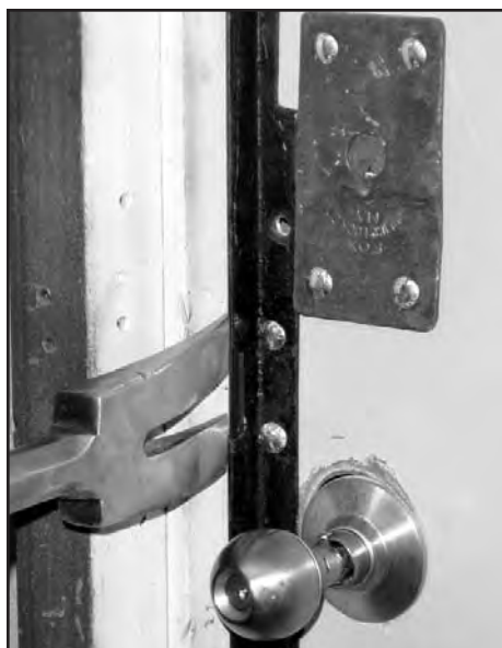
Figure #2--Place the fork (bevel to door) between the angle iron and the door frame, six inches above or below the lock.
