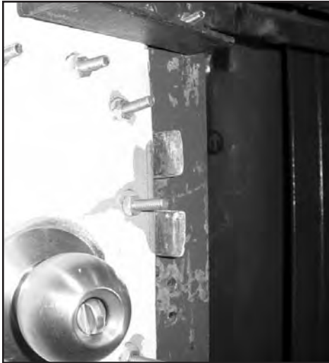
Figure #7--The tips of the Halligan tool are locked on the inside of the door frame.
