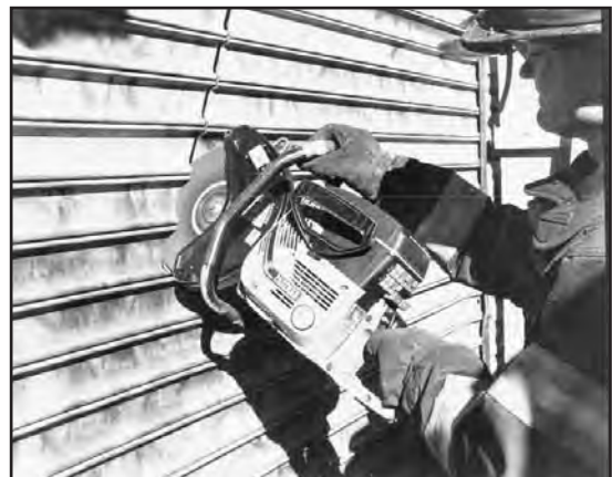
(Right) The first cut is made at an angle from the top to the bottom of the gate.
