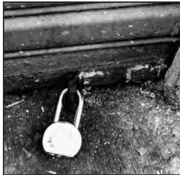
Cutting the American 2000 series lock with a power saw. Note: Cutting the lock is the most reliable and common procedure. photo by Captain Robert Morris
