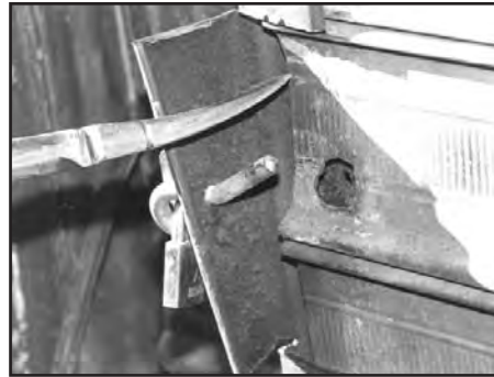
(Left) Bend the rail and pin out.
