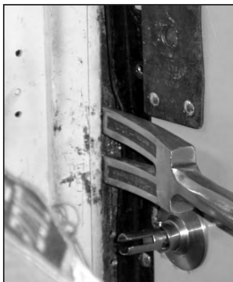
Figure #5--Push tool sharply toward the door, using the angle iron as a fulcrum, forcing the door in. This move pushes the door in and may force it but, at the very least, will make it easy to drive the fork in.
