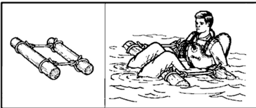
Figure 17-8. Log flotation.
