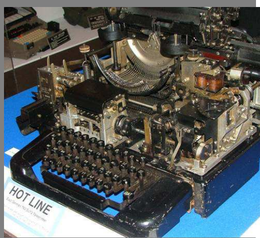
The East-German T-63, used on the US-USSR hotline, together with the ETCRRM one-time tape mixer. Image courtesy National Security Agency. © NSA.
