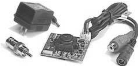
They are also useful for back-up surveillance in installations where the primary CCTV equipment is of a more traditional nature, i.e. standard cameras. In this case Covert Cameras can operate
